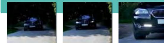
Without DRL With low beam on With LED DayLightGuide
