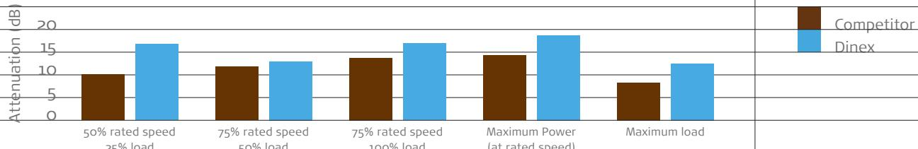
Sound attenuation is the ratio between the radiated sound power level of the exhaust system, with and without the silencer installed. An overall sound attenuation of 10 dB will by a human ear be perceived as halving of the noise level.
