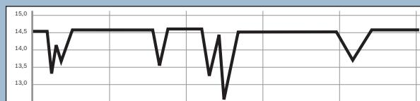
Characteristic: Large number of start operations, resulting in higher load on the battery
