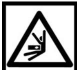
Sign informing about the possibility of crushing when a person stays between the tractor tie rods and how to avoid the risk by not staying near tie rods when controlling the hydraulic lift (label located on the log grapple body surface).
