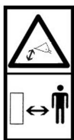
A sign informing about the mechanical risk of being crushed by the grapple and how to avoid the hazard by keeping a safe distance from the grapple (label located on the side plane of the grapple body).
