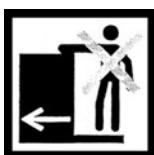
Sign informing about the prohibition of climbing onto the log grapple while working, especially during loading (label located on the grapple body surface).
