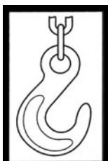
Sign informing about the locations used for lifting the machine with lifting devices (label located on the log grapple body surface).
