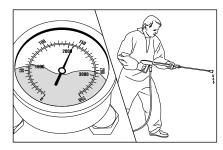
The stainless steel pressure gauge shows full pressure, but from the nozzle comes only little water or no water at all.
