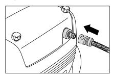
11. Connect the water hose to water inlet sieve. The high pressure cleaner may be connected to a water mains (1-10 bar pre-pressure) with either cold or hot water (up to 60 °C). The large quadro series provides the opportunity of sucking in water out of a container (see direct suction).
