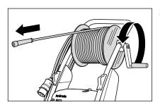
5. Unwind high pressure hose straight and without nooses. For high pressure cleaners with hose drum please release fixing of hose drum at first and fully uncoil it after that. (When extending the high-pressure hose please consider the maximum length of 20 m!)
