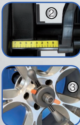
(1) Side holder for centering cones and gauge (2) Integrated distance measurement (3) Quick release nut \varnothing = 36 mm (4) The new diagonal ergonomic design is user friendly and has 11 storage compartments included (5) Digital Display
