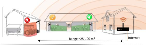
(2)WiFi Router->farmCam IP with antenna outside the wall
