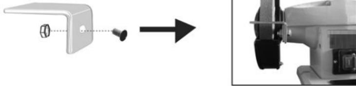
Fit the tool rest, over the wheel guard securing bolt and secure in place with the bolts supplied. Adjust it so there is approximately 2 mm between the grinding wheel face and the tool rest.
